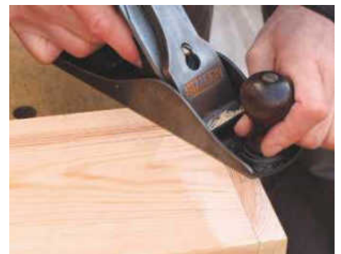
STEP 10. When the glue has dried, plane the end-grain flush at the top of both side panels
